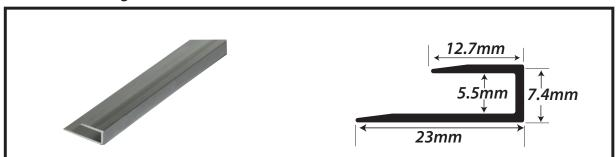
Floating Floor Box Edging are used to finish off the edges of your new timber floor where it joins other floor coverings like carpet, vinyl, ceramic tiles, or timber. They are also designed to cover expansion gaps in doorways and within larger floor areas. vinyl on most substrates.
